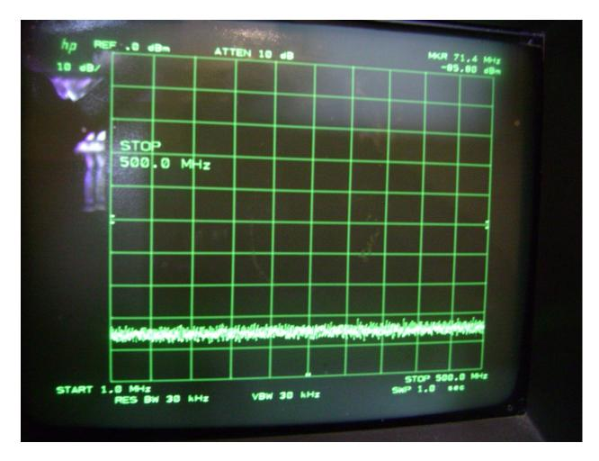
THIS IS A SPECTRUM ANALYZER PLOT SPANNING 1 MHZ TO 500 MHZ WITH NO INPUT ON THE TV END OF THE COAXIAL CABLE. NOTE THE LEVEL OF THE NOISE FLOOR IS ROUGHLY -85 DBM.
