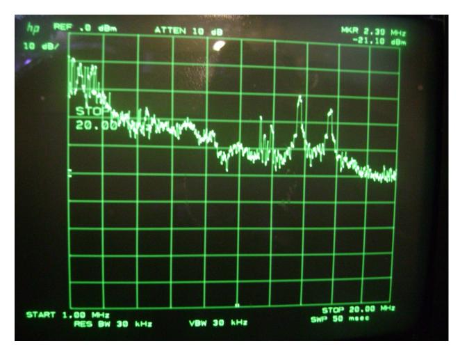
THE NEXT PLOT PRESENTS A MEASUREMENT OF THE INTERFERENCE (CONDUCTED EMISSIONS) FROM 10 MHZ TO 20 MHZ. ACCOUNTING FOR THE TRANSFER FUNCTION OF THE CURRENT PROBE, THE TWO PEAKS AT ROUGHLY CENTER ARE 90 DB ABOVE THE BASELINE. EVERYTHING IS AT LEAST 60 DB ABOVE THE BASELINE (WITH THE TRANSFER FUNCTION ACCOUNTED FOR).
